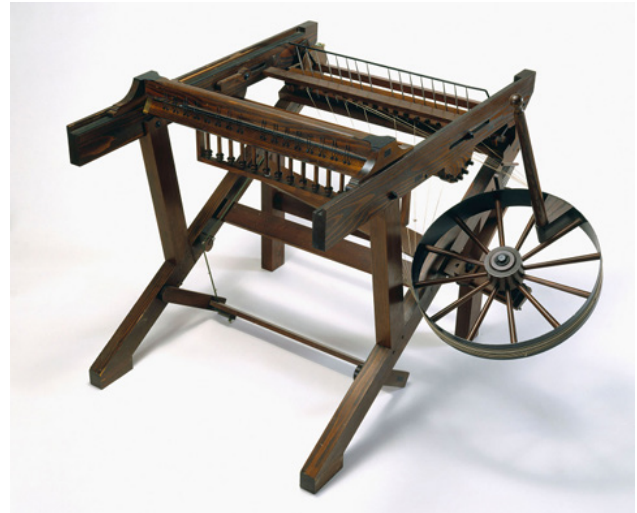
Figure 3 A sixteen-spindle spinning jenny, reconstructed from James Hargreaves' 1770 patent drawings, Science Museum, London, 1970-0174. Source from the Science Museum/ Science and Society Picture Library.
