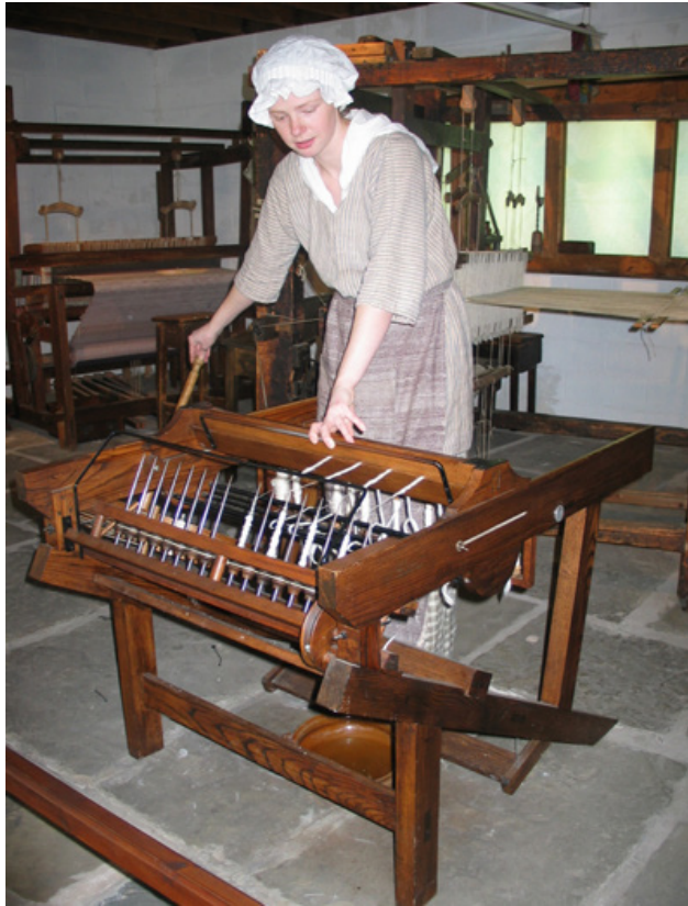
Figure 1 Reconstruction of a sixteen-spindle spinning jenny, based on the specification drawings in James Hargreaves' 1770 patent. Source from Styles
