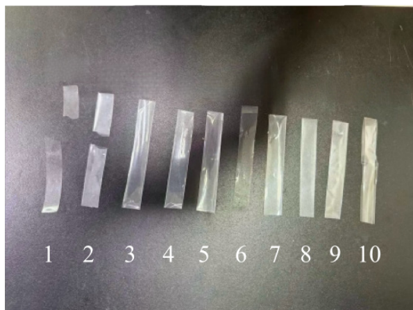
Fig. 1. Photos of PP Film Before and After Electron Beam Irradiation with Different Doses
