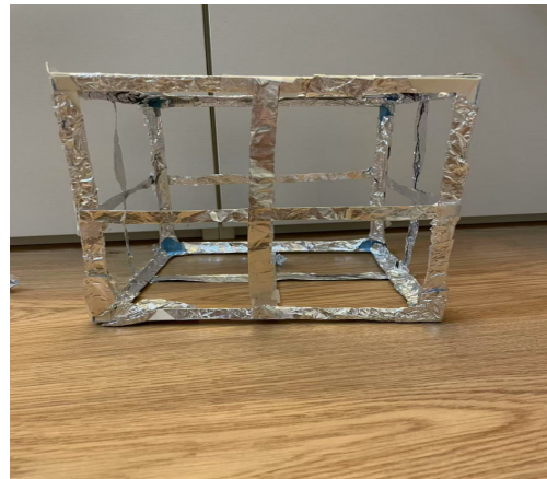
Figure 5 (a): model of the frame of the cage presents in 3.2.4 and its size. (b): Faraday Cage used in 3.2.4.
