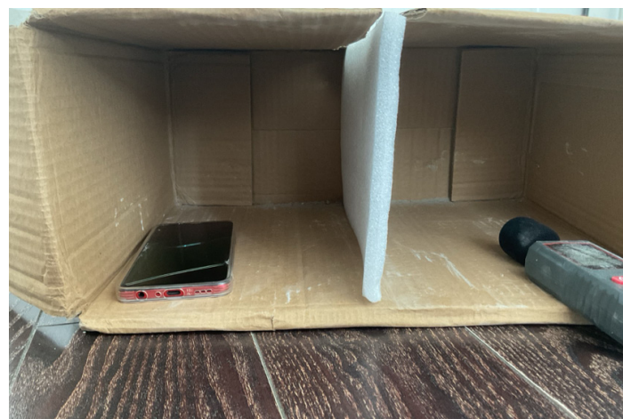
Figure 3.2. The setup of the experimental apparatus using foam board.
